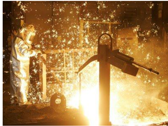
Pouring molten steel. © United States Steel Corporation.
